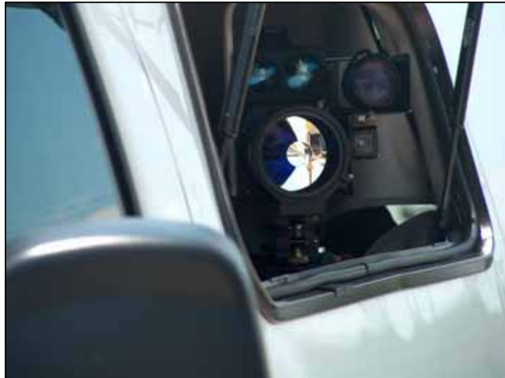
<Figure 13> Laser Speed Gun and Camera Viewed from Outside Van (35)
