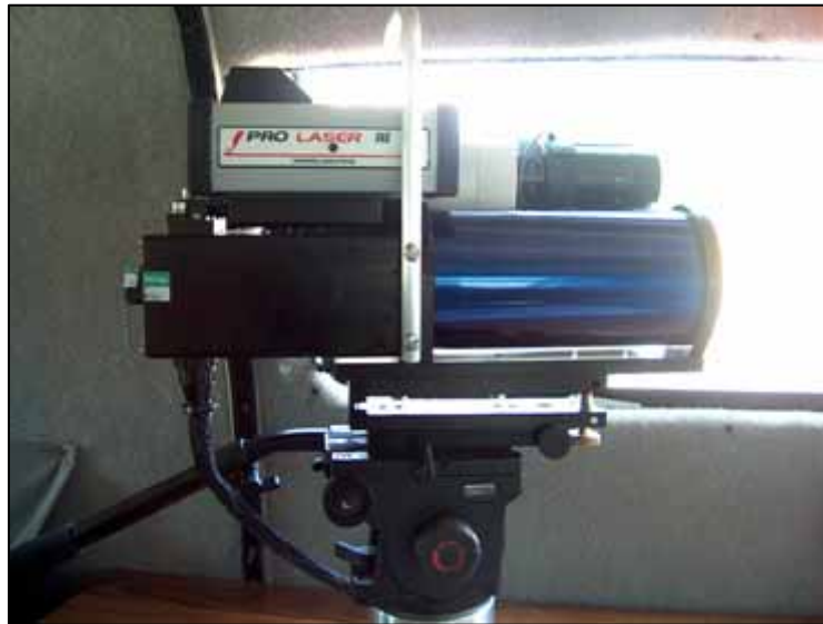
<Figure 12> Laser Speed Gun and Camera (35)
